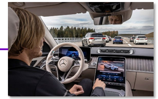
MERCEDES-BENZ LEVEL 3 DRIVE PILOT (specific highways, only up to 60 km/h)
